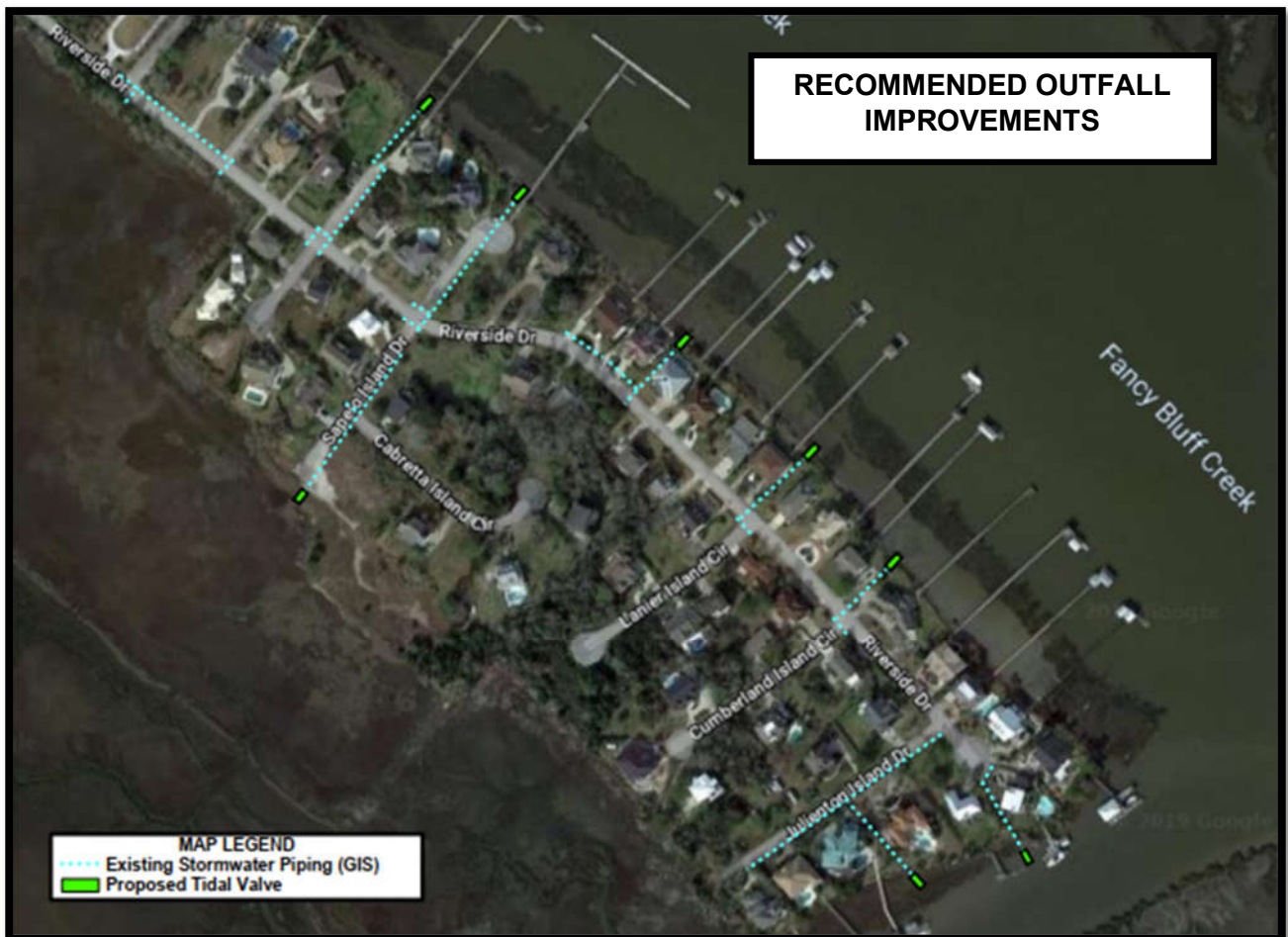
Figure 37: Riverside Neighborhood Recommended Outfall Improvements
