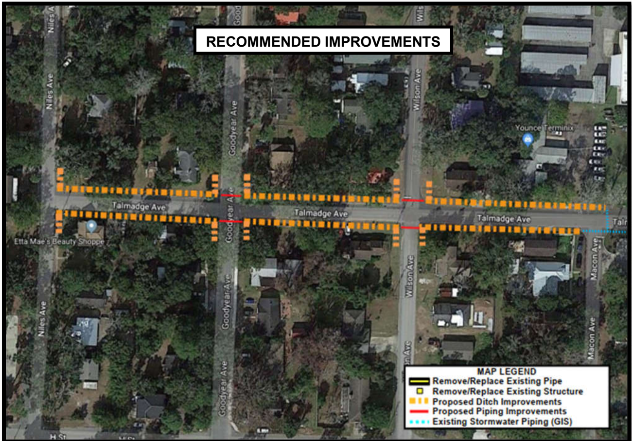
Figure 27: Talmadge Avenue Ditches Recommended Improvements
