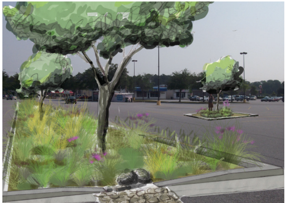
Proposed parking lot island with vegetated bioswale
