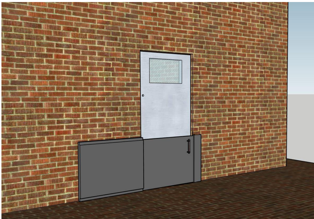
Flood proofing for commercial buildings can include the temporary addition of large shields on primary entrances (above) or more permanent shields on rear doors not readily visible from the street (below).
