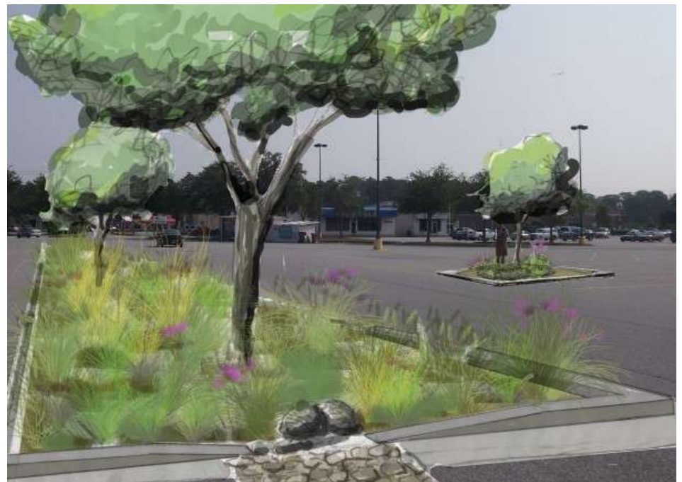
Proposed parking lot island with vegetated bioswale
