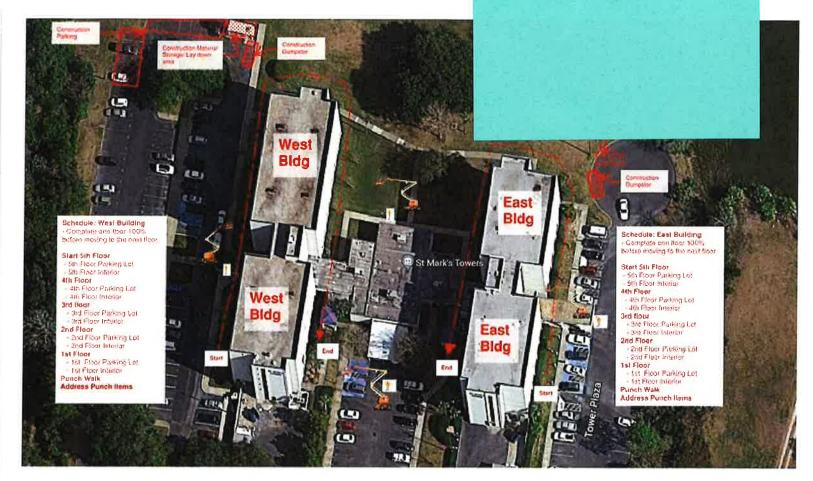
The approach is to begin on the top floor of the building, completing the window and PTAC replacement concurrently, for the entire floor before moving to the floor below. The buildings can be worked on concurrently or sequentially, per the Client's preference.
