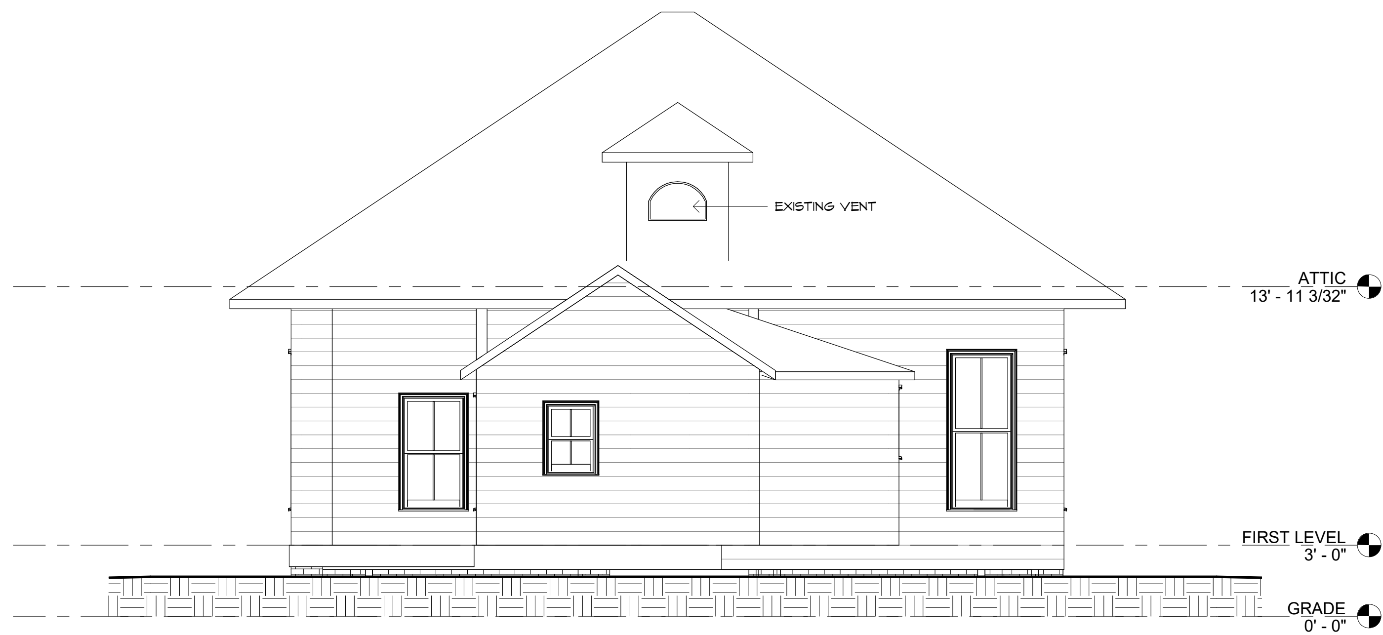
④ REAR ELEVATION - EXISTING 1/4" = 1'-0"
